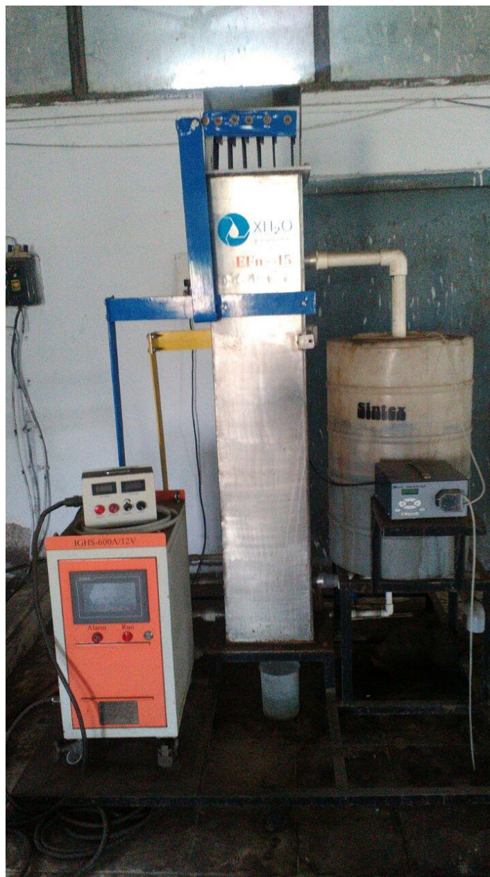
IMAGE: PILOT SCALE ELECTRO FENTON
