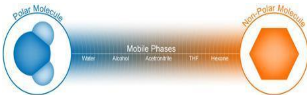
Figure: 3 Mobile phase chromatographic polarity spectrum
