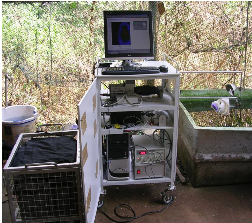
Fig.4. Experimental setup of LIF imaging of corals using LIMFIS at CMFRI, Vizhinjam
