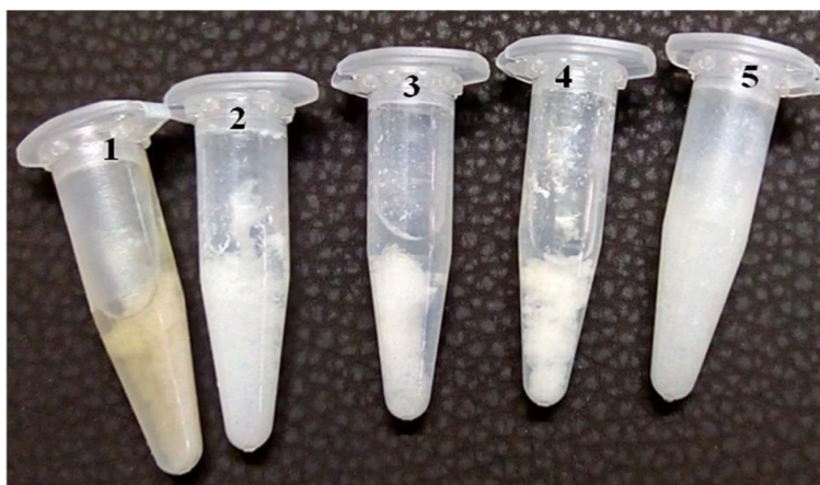
Figure 11: Milk clotting activity of the purified protease. 1. Crude sample, 2. 0-60% fraction, 3. Purified protease, 4. Positive control, 5. Control.
