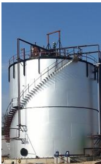
Figure 2: Hybrid anaerobic reactor (Kaashyap Envergy Reactor)
