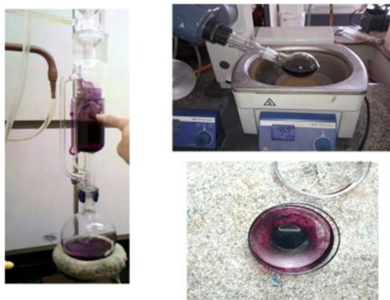
Figure 1. Soxhlets method of extraction procedure and concentrated fruit extract in petri plate.
