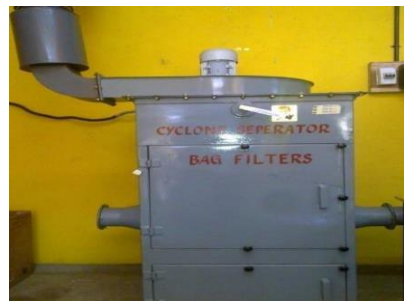
Fig 12. Working place of dismantling, cyclone chamber, Connection with bag filters
