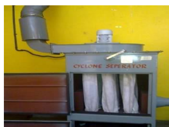
Fig 13. Bag installed in cyclone chamber and cyclone bag filter with stack
