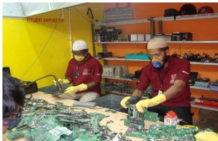
Fig 7. (a), (b) and (c) Dismantling of computer component and PCBs
